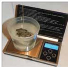
Figure 2 - Measurement of sample volume by freely suspending and submersing specimen in a water-filled and tared plastic container. Balance readout is equivalent to volume of object in  $\text{cm}^3$ .
