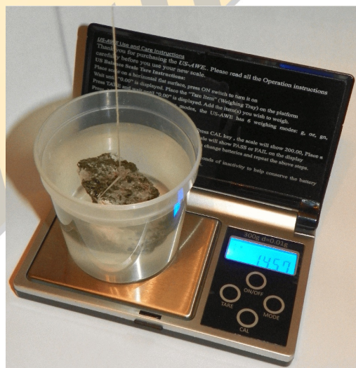
Figure 2.4 - Mineral Density Quick Test using the single pan hydrostatic method and a load cell balance
